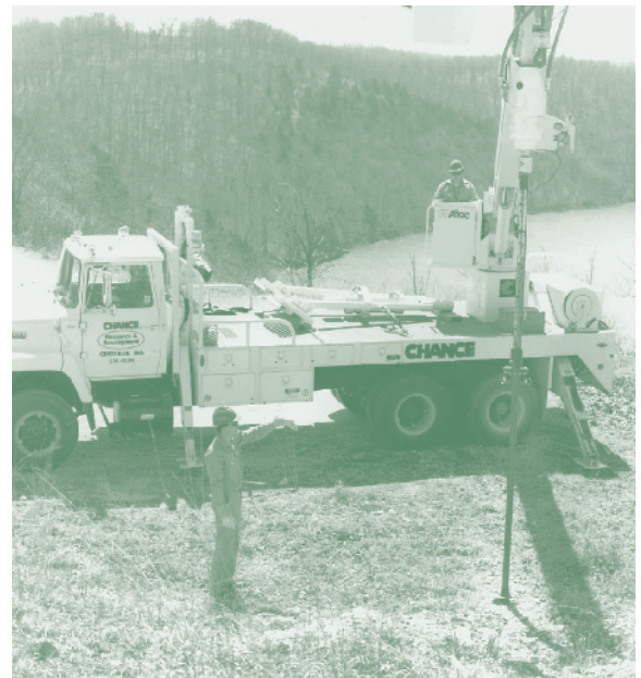
Chance has a full fleet of anchor testing equipment to help utilities plan their anchoring requirements.
